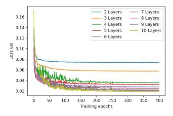
Figure 4: **Performance of the CNN sorter with respect to the depth of the CNN**. Value of the cost function during the training of multiple CNN sorters with a number of layers varying from 2 to 10. The model performances saturate for models with 8 layers or more.
